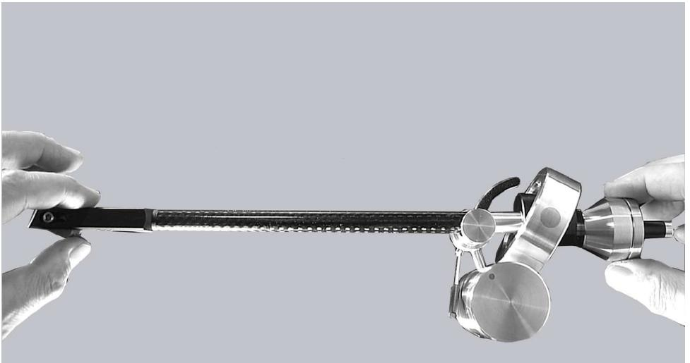
Now you are ready to mount your cartridge. Unscrew the head shell plate and install your cartridge with the supplied non-magnetic M2.5 screws to the threaded holes. Choose the length of the screw that will fit to your cartridge and not stick out the top of the plate when fixed. Put the head shell plate back to the arm wand and tighten it lightly, so that it still can be moved back and forth.
